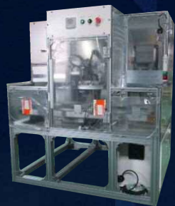
光通信コネクタ組立装置 Fiber optic connector and adapter assembling equipment
